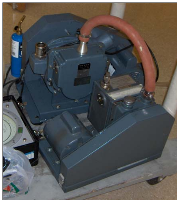
Figure 16. Piggy-Backed Vacuum Pumps
