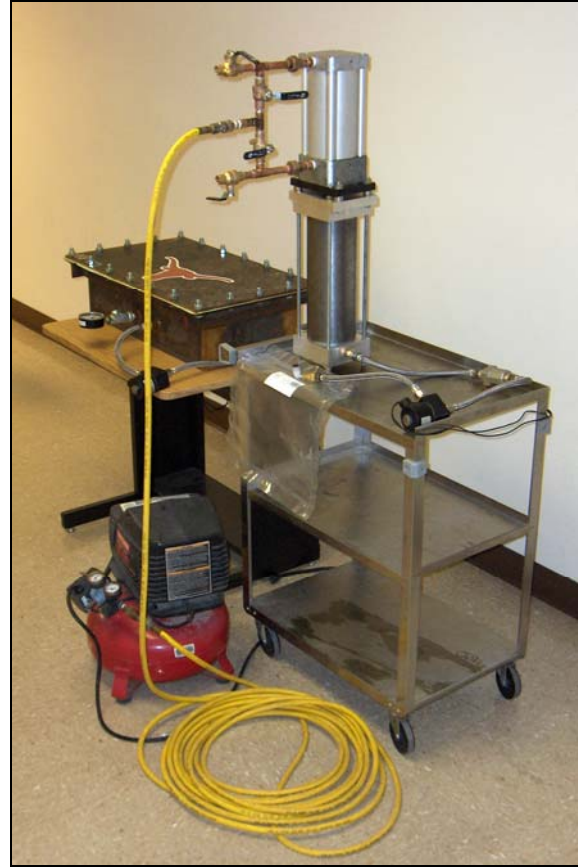
Figure 11. Extra-Terrestrial Water Extraction Test Apparatus
