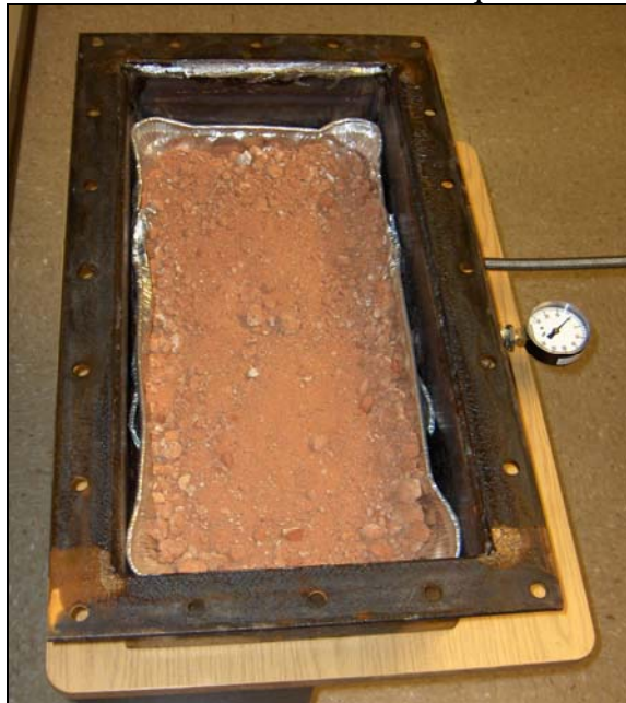
Figure 13. Sublimation Chamber with Mars Regolith Simulant
